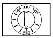
After using the refrigerator for 24 hours, adjust the thermostat to the setting that is best suited to your needs. Turning the thermostat to **OFF** stops the cooling cycle but does not shut off power to the refrigerator.
