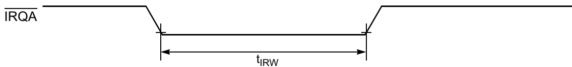
Figure 10-6 External Interrupt Timing (Negative Edge-Sensitive)
