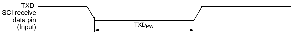
Figure 10-16 TXD Pulse Width
