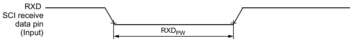
Figure 10-15 RXD Pulse Width
