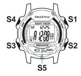
**S1**= Start / Stop button S2= Lap/ Reset button. S3= Mode button.
