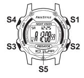
**S1**= Start / Stop button S2= Lap/ Reset button. S3= Mode button. **S4**= Light button.
