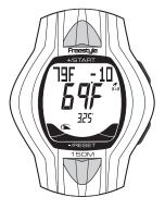
To adjust the values and offset press down S1 for at least three seconds until the temperature unit flashes. Select between FHT for farenheit or CEL for celsius. Pressing S2 moves you on to the offset setting.Press S3 or S4 to adjust the reading.
