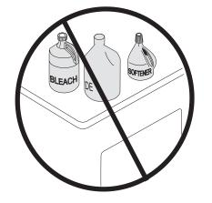
Do not store or place laundry products on top of dryer at any time. They can damage the finish or controls. **WARNING** To reduce risk of fire or serious injury to persons or property, comply with the basic warnings listed in *Important Safety Instructions* and those listed below.
