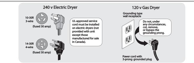
Avoid fire hazard or electrical shock. Do not use an adaptor plug or extension cord or remove grounding prong from electrical power cord. Failure to follow this warning can cause serious injury, fire or death.
