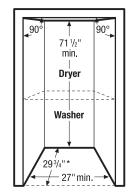
Stacked Units in Recessed or Closet Installation For detailed stacked installation, refer to instructions included with Stacking Kit or on web. Note: Stacked installation requires modified utility hookup locations for dryer. For details, refer to Product Installation Guide on web.
