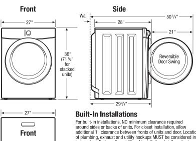
additional 1" clearance between fronts of units and door, Location of plumbing, exhaust and utility hookups MUST be considered in built-in installations. For additional installation details, refer to Product Installation Guides on web
