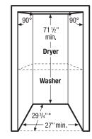
Stacked Units in Recessed or Closet Installation For detailed stacked installation, refer to instructions included with Stacking Kit or on web. Note: Stacked installation requires modified utility hookup locations
