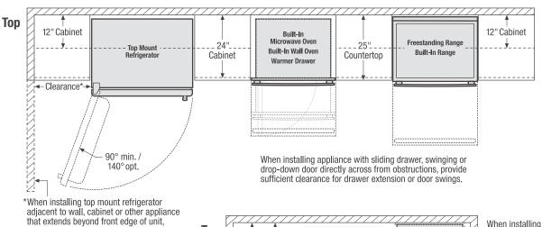
\*When installing top mount refrigerator adjacent to wall, cabinet or other appliance that extends beyond front edge of unit, 20" minimum clearance recommended to allow for optimum 140° door swing, providing complete crisper access and removal. (Absolute 3" minimum clearance will ONLY allow for 90° door swing which will provide limited crisper access with restricted removal.)
