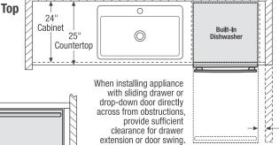
appliance with sliding drawer or drop-down door adjacent to wall, cabinet, or other obstruction that extends beyond front edge of appliance, allow 2" minimum clearance between drawer or door and obstruction.
