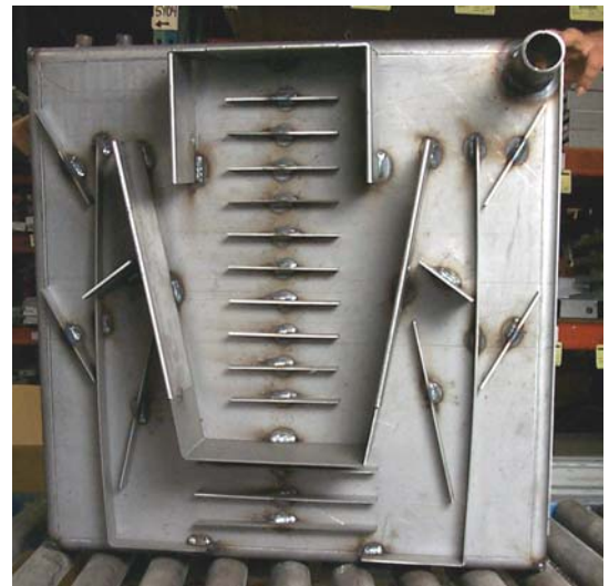
Heated air is drawn across the bottom of the 24G frypot with a blower-driven draft system.
