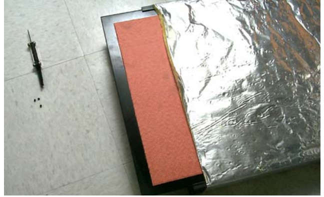
Fig. 12: The heater plate slides from the insulation.
