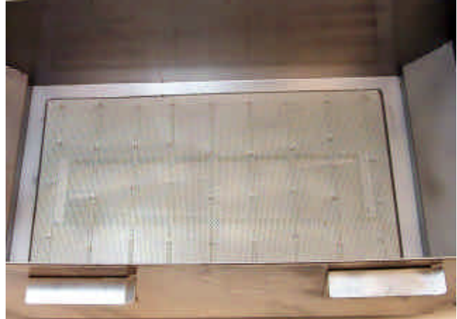
Support grid properly placed in filter pan.
