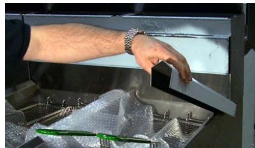
Figure 7. Install joiner strip(s) after fryers are connected.
