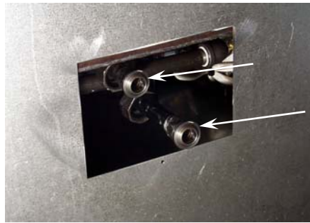
Figure 5. Oil return and rinse-line (where applicable) connections.
