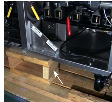
Figure 1. Remove pallet supports (arrow) before removing fryers from pallets.
