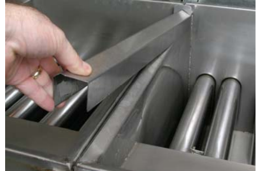
Removing the joiner strip.
