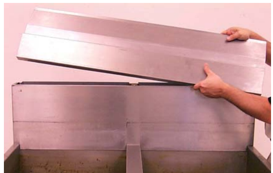
Removing the basket hanger from the flue cap.
