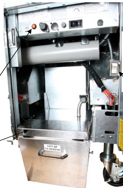
Figure 4: The assembled melter is shown in position.
