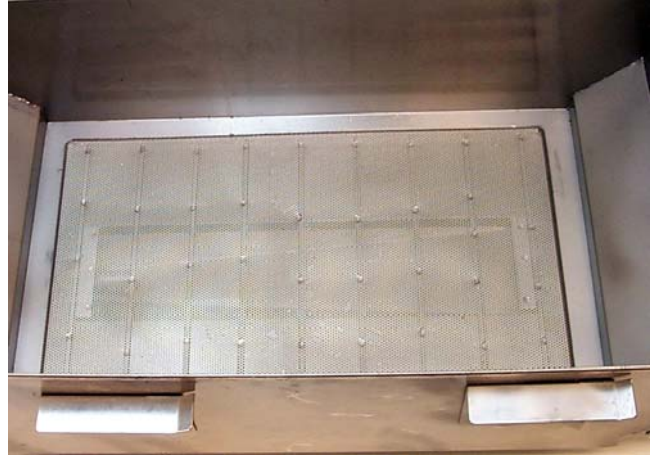
Support grid properly placed in filter pan.
