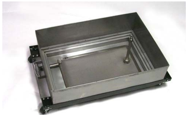
Filter leaf properly positioned in filter pan.
