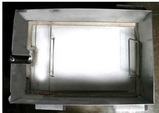
The hold-down ring is shown resting on the filter pad. The notches in both are turned toward the pick-up tube.
