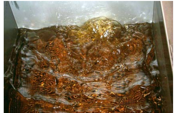
Allow the oil to bubble for 15-30 seconds after the filter pan is empty to clear the oil-return lines.
