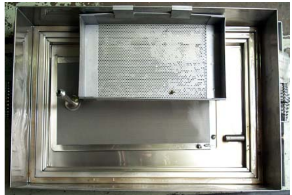
Placing the crumb screen.
