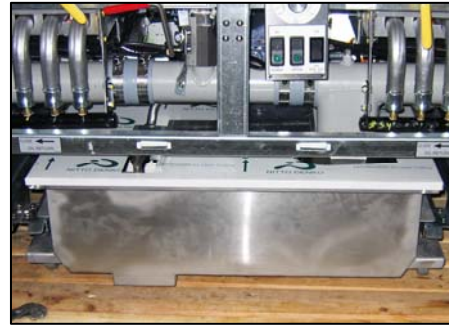
Figure 1. Remove the filter pan by pulling it out from underneath the fryer.
