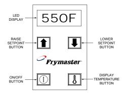
*To change the display from Fahrenheit to Celsius:* Unplug the unit, then press and hold the **U** button as the unit is plugged back in.
