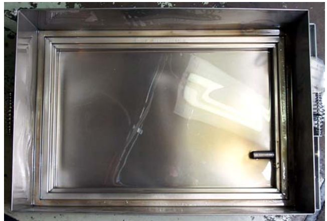
Filter pan with cover removed.
