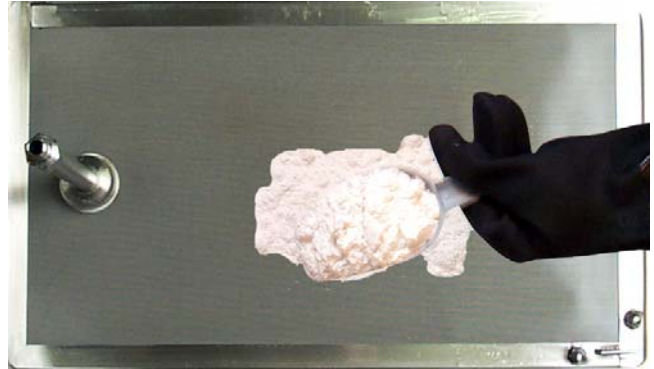
Applying filter powder to filter-leaf.
