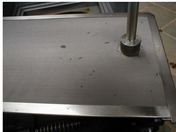
Optional filter-leaf used in place of filter paper.
