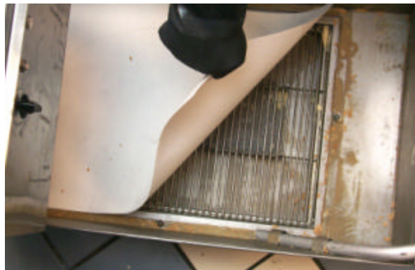
Solidified shortening build-up around and in nipple-pipe assembly.
