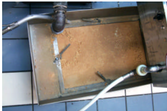
Scrape excess sediment from top filter paper sheet after filtering.
