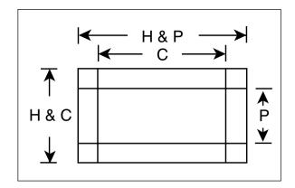
Even when anyone of the P/H/C print format has been selected, the size of the photograph on the film remains the same (16.7 x 30.2 mm). Print format selection will record the print format for each frame and the exposure will be printed within the ranges shown in the above illustrations.
