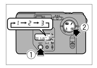
Hold down the SHIFT button ① and press the ③ mark on the multi-operation button ② to illuminate only the ③ guide lamp. Continue to press the ⑤ mark to select the number of required self-timer exposures (maximum of 3.) The self-timer exposure count displayed in the LCD will be selected when the SHIFT button is released, and the guide lamp will be extinguished.
