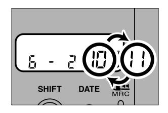
The exposure film is rewound once (the exposure counter also counts back 1 frame) then returned to the last position. The exposure counter also returns to its original value, and the title is changed.
