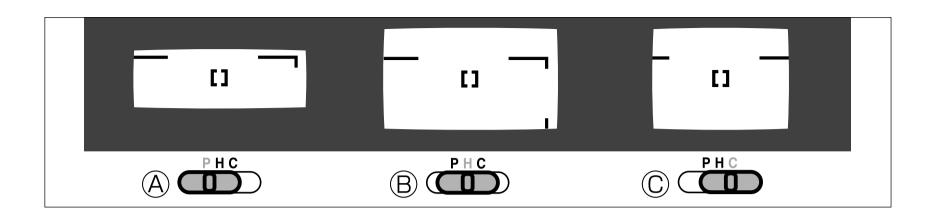
The view through the finder will change to the style of photographs shown when the format selector is operated. The angle of the exposure will not change.
