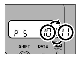
The film is first rewound (the counter is reset to frame 1), then advanced to its original position (the counter is also advanced), and the print quantity is changed.
