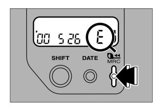
Press the mid-roll change button to rewind the film when the cartridge is to be ejected in the middle of the roll. Do not remove the cartridge until "  $\xi$  " is displayed in the exposure counter and the rewind motor has ceased to operate.
