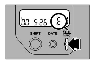
Press in the mid-roll change button. The film counter will display as it subtracts from the number of exposed frames. When rewinding is completed, "  $\xi$  " will be displayed by the film counter.
