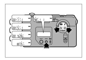
Press the multi-operation button's UP or DOWN button to correct the numeral blinking on the LCD. Adjustable items are as follows.
