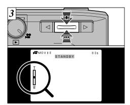
The "▲( 📭 )" and "▼( 👀 )" button control the digital zoom. A zoom bar is shown on the LCD monitor.
