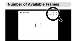
The number of available shots is displayed on the LCD monitor in the position shown in the figure at left.
