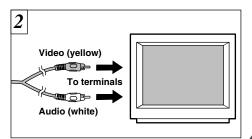
Plug the other end of the cable into the audio/video input socket on the TV. Then switch the camera and TV on and take pictures or play back images as you would normally.
