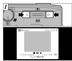
Use "◀" and "▶" button to select the movie file. The screen used for movie appears on the LCD monitor.
