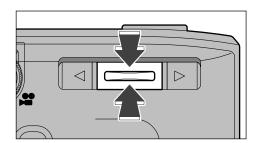
Pressing "▲( 📭 )" when the file size is set to "1280  $\times$  960" or "640  $\times$  480" selects digital zoom mode. However, this is only possible when you are using the LCD monitor to take pictures.
