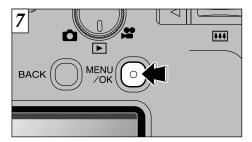
To reset the print settings, press the "MENU/OK" button to display the image for which you want to reset the settings.
