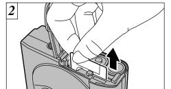
Taking care that the batteries do not fall out of the camera, grasp the SmartMedia and pull it out.
