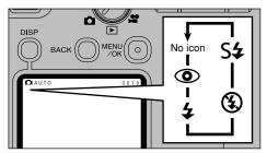
You can choose from 5 flash modes to suit your shot. Each time you press the "4" flash button, the flash mode shown on the LCD monitor changes from Auto flash (no icon displayed) to "o" to "≰" to "S≰". The last mode displayed is the selected mode.
