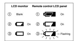
Check the battery level warning when you switch the camera on.
