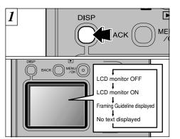
In Auto mode, the LCD monitor display changes each time you press the "DISP" button. Press the "DISP" button to display the "Framing Guideline".
