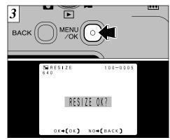
A confirmation screen appears. To proceed, press the "MENU/OK" button. The resized image is recorded as a separate file.
