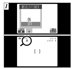
You can set the self-timer when the photography mode is set to "□A" or "□M". When you select "ON", the "" icon appears on the LCD monitor.
