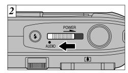
To use the camera for audio, slide the POWER switch to "AUDIO". Note that this only turns the camera on for audio playback.
