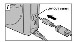
Switch off the camera and TV. Plug the A/V cable (accessory) into the A/V OUT (audio-visual output) socket on the camera.
