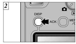
To take pictures using the viewfinder (excluding Macro Photography), To use the LCD monitor to take photographs, press the "DISP" button to switch the LCD monitor on (→P.29).
