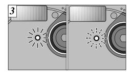
The self-timer lamp lights for 5 seconds and then blinks for 5 seconds, then the camera takes the picture.
