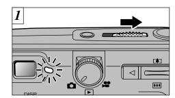
To turn the camera on or off, slide the POWER switch to " POWER ".
