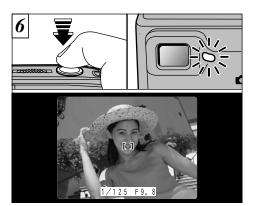
Press the shutter button down half way. The image is focused when the AF frame on the LCD monitor becomes smaller and the shutter speed and aperture setting appear (and the green viewfinder lamp stops blinking and remains lit).
