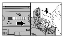
Switch the camera off and replace the SmartMedia.
