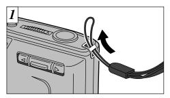
Pass the loop of thin cord on the end of the strap through the strap mount.
