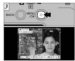
When you press the "MENU/OK" button, the cropping settings are determined as shown in the image on the LCD monitor.
