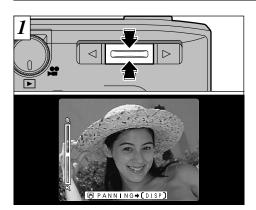
Pressing "▲( 📭 )" and "▼( 🚻 )" button during playback zooms in and out on (enlarges and reduces) the still image respectively. When you use this function, a zoom bar is displayed.
