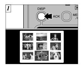
Pressing the "DISP" button twice switches to the multi-frame (9-frame) display.
