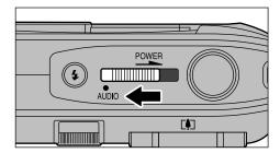
Note that this only turns the camera on for audio playback with the remote control connected.
