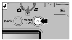
Press the "MENU/OK" button to erase the displayed image. When erasing is complete, the next image appears and the "[FRASE OK?]" message is displayed.
