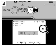
When the "MENU/OK" button is pressed, the 4 image is protected and the "em" icon appears on the right of the screen. To remove the protection, press the "MENU/OK" button again.
