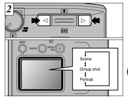
Use the "◀" and "▶" buttons to select one of the three framing guidelines. The framing guideline help you to compose your shot when you are taking pictures using the LCD monitor.
