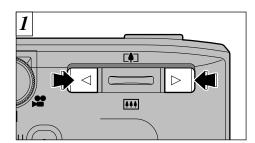
You can fast forward through the frames by holding down "◀" or "▶" button for about 3 seconds during playback.
