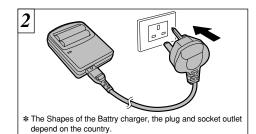
Plug the charger into a power outlet to begin charging. Battery charging will be completed in about 13 hours, but the power lamp remains lit. Unplug the battery
