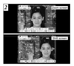
You can alternate between the Zoom and Shift screens by pressing the "DISP" button. Using the Zoom screen:
