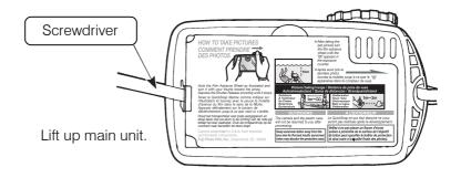
3. Remove the main unit by rotating the bottom part outward.
