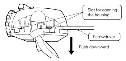
2. After removing the rear cover, insert the screwdriver into the slot on the side opposite the strap and lift up the main unit.
