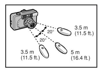
The coverage of the remote controller is up to approx. 5 m (16.4 ft.) when used directly in front of the camera, and up to approx. 3.5 m (11.5 ft.) when used at a vertical or horizontal angle of  $20^{\circ}$ .
