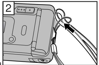
Do not use a strap made for cellular phones or similar electronic products. These straps are usually too light or weak to hold your camera securely. For safety, use only straps designed for cameras.
