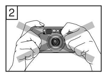
Make sure that nothing is in front of the lens, the flash, the AF (Auto-Focus) windows or the AE (Automatic exposure) light sensor.
