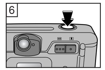
Press the shutter release button down completely.
