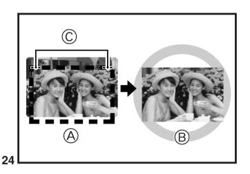
When taking close ups, an area seen through the viewfinder and the area seen by the lens and actually photographed will be different. This is because the viewfinder and lens are not in the same position, a difference known as "parallax". The parallax correction guides indicates the difference between what the viewfinder sees and what the lens sees when the picture is taken.
