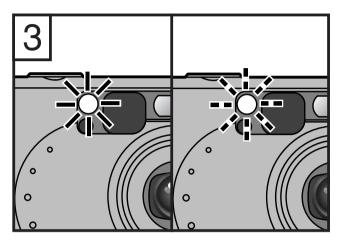
After the self-timer lamp remains lit for approx. 7 seconds, it blinks for approx. 3 seconds, and then the shutter is released. When taking consecutive exposures, the shutter is released the set number of times at an interval of between 3 and 6 seconds.
