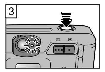
With the AF frame positioned over the subject, press down the shutter release button halfway to set the Auto-Focus lock.
