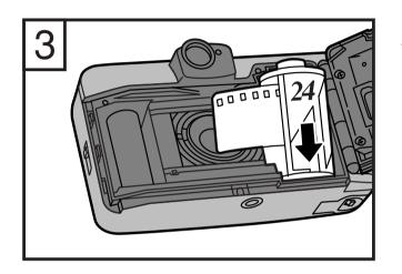
Insert the roll of film. Keep the long end of the spool in the film cassette at the top of the film compartment as shown in the drawing.
