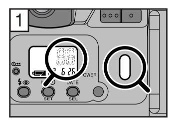
Check that there is not a film in the camera and that the exposure counter is not displayed.
