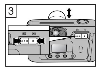
To use the zoom lens, press the [4] mark until you see the composition you want in the finder. Pressing the [44] mark will set the lens at the shorter focal lengths to obtain wide-angle coverage.
