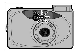
The self-timer lamp will begin to blink approximately seven seconds after being illuminated, and the shutter will be released approximately three seconds after that.
