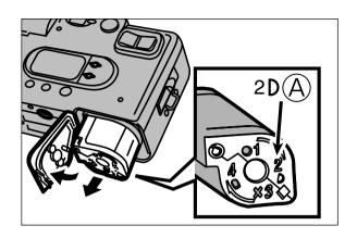
Remove the cartridge and sign sure the sign D appears white.
