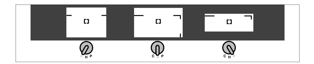
The view through the finder will change to the style of photographs shown when the print format switch is operated. The angle of the exposure will not change.
