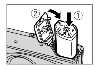
Drop the cartridge ① into place and then close the cartridge cover ②.
