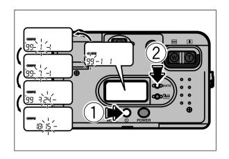
Press the DATE button to select the next number blinking in the order Year  $\rightarrow$  Month  $\rightarrow$  Day  $\rightarrow$  Hour  $\rightarrow$  Minute. Press the  $\circ$  button  $\circ$  to correct the numerals blinking in the liquid crystal display. If you press the DATE button  $\circ$  at this time, the blinking numerals to be corrected will change in sequence from Year  $\rightarrow$  Day  $\rightarrow$  Hours  $\rightarrow$  Minutes.
