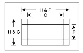
Even when anyone of the C/H/P print format has been selected, the size of the photograph on the film remains the same (approx. 17 x 30mm). Print format selection will record the print format for each frame and the exposure will be printed within the ranges shown in the above illustrations.
