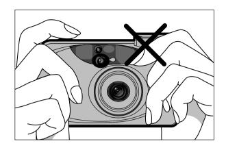
Ensure that fingers or the camera strap are not obscuring the lens of flash assembly.
