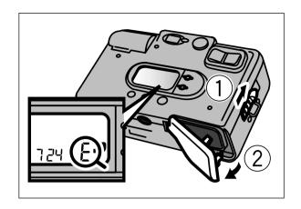
When the exposure counter shows " E " and the motor stops, move the film cartridge compartment cover release knob as indicated in ①, in the direction indicated in ②, and open the film cartridge compartment cover.
