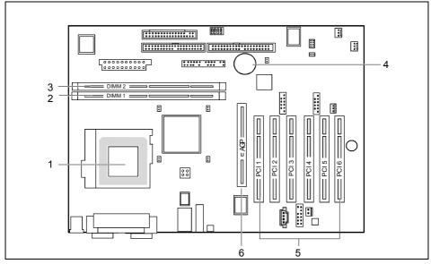
1 = Socket for processor with heat sink
