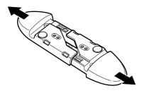
2 Install the feet on the main unit of the personal computer. Secure them in the screw holes on the back of the feet with screws.
