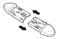
2 Install the disassembled foot on the main unit of the personal computer. Secure it in the screw hole on the back of the foot with a screw.
