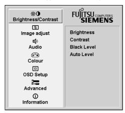
The first symbol (*Brightness/Contrast*) is highlighted. In the right-hand part of the display the associated functions are shown.
