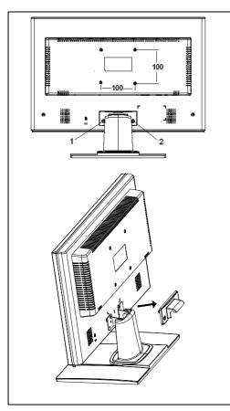
Remove the screws on the rear of the monitor.
