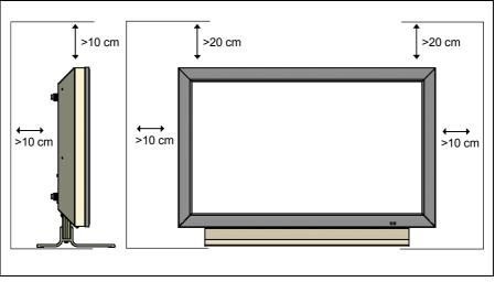
When installing the TV in niches, maintain the minimum distance for sufficient ventilation of the device: 10 cm from the side and back, 20 cm from the top.
