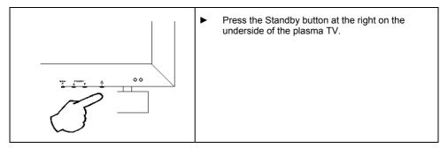
From the indicator at the lower right on the front of the plasma TV you can recognise whether the device is in operation, in the standby mode or switched off.
