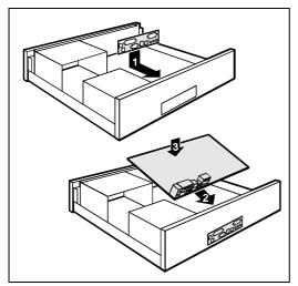
Should no suitable connection field be provided in the case, then you must install the connection field (1) provided.
