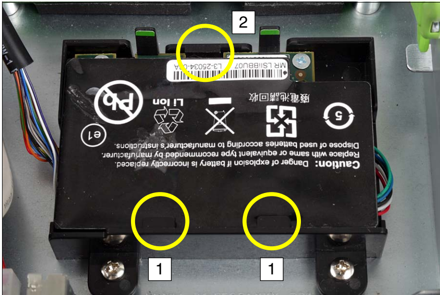
Figure 32: Installing the iBBU
