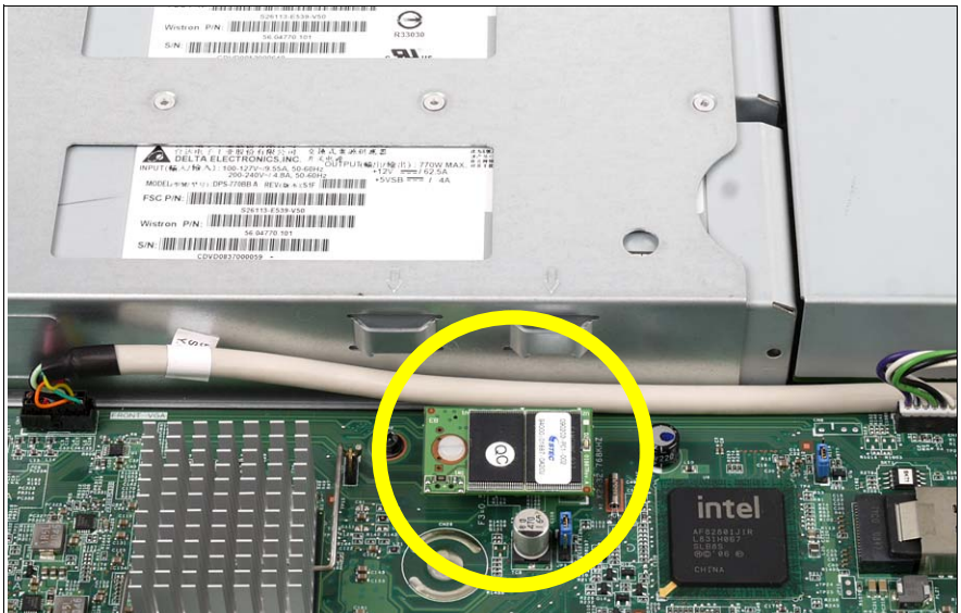
Figure 35: Position of the uSSD on the system board
