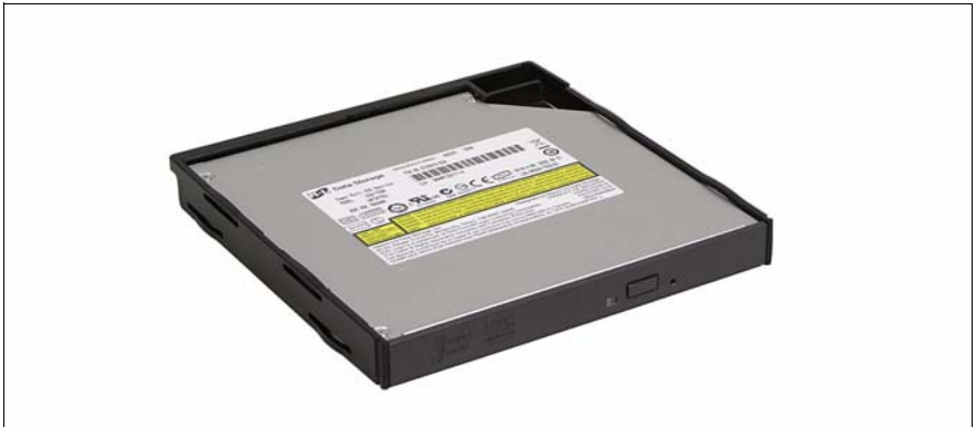
Figure 18: The DVD drive ready to be installed
