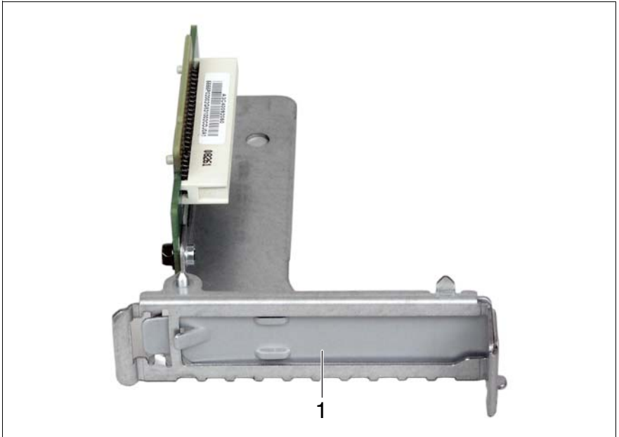
Figure 26: Riser card holder #2 with riser card
