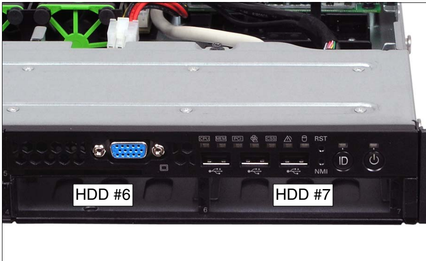
Figure 24: Installation positions of additional HDD modules
