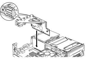
9 Install the upper cover and connect LAN and modular cables.
