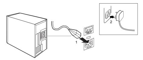
Plug the system unit's power cable into the system unit (1) and then into the grounded mains outlet (2).
