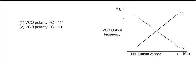
Note: Give attention to the polarity for using active type LPF.
