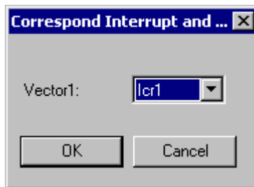
Figure 4.5-11 Correspondence between External Interrupts and ICRs
