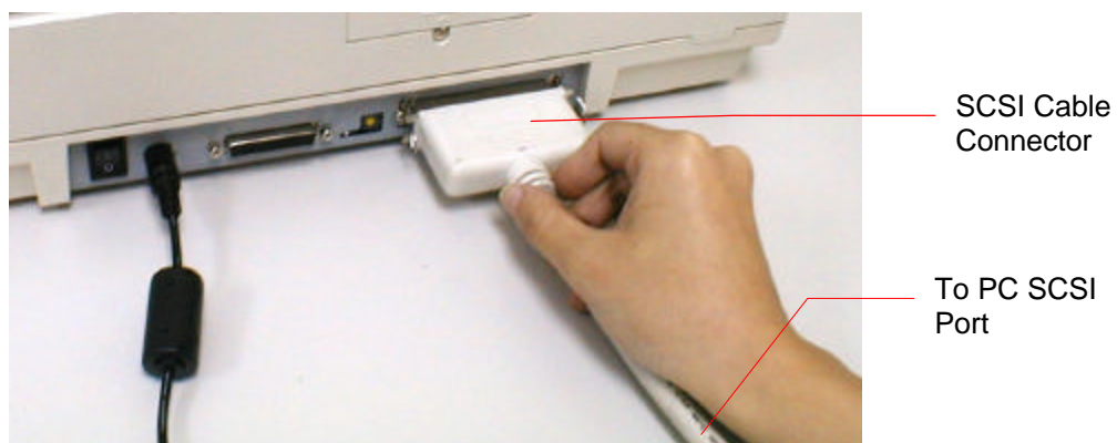
Figure 2-9 ScanPartner 620C SCSI Cable Connection
