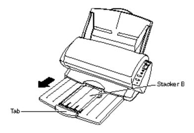
2) Insert a finger into the dent at the center of the stacker, then lift and pull the Stacker B.
