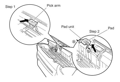
4) When mounting a new pad unit, push the pick arm downward with one hand while mounting the pad unit with the other hand.
