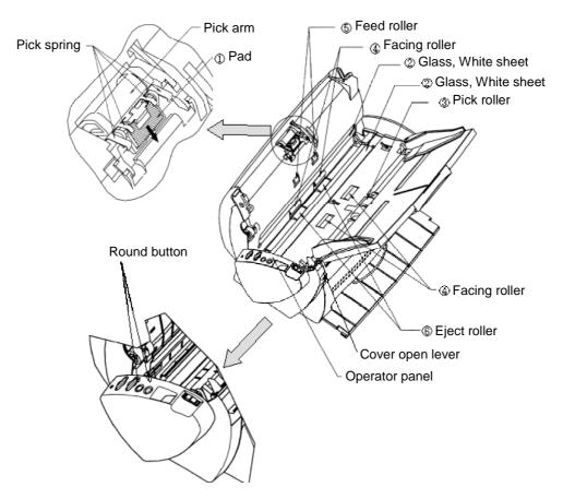
Parts to be Cleaned on the Automatic Document Feeder
