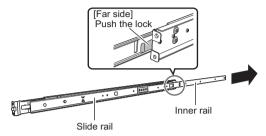
**4** Attach the inner rails on the right and left side of the server.
