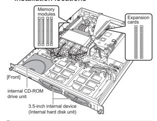
After installing internal options, check that the order and place of installation are correct and cables are correctly attached.
