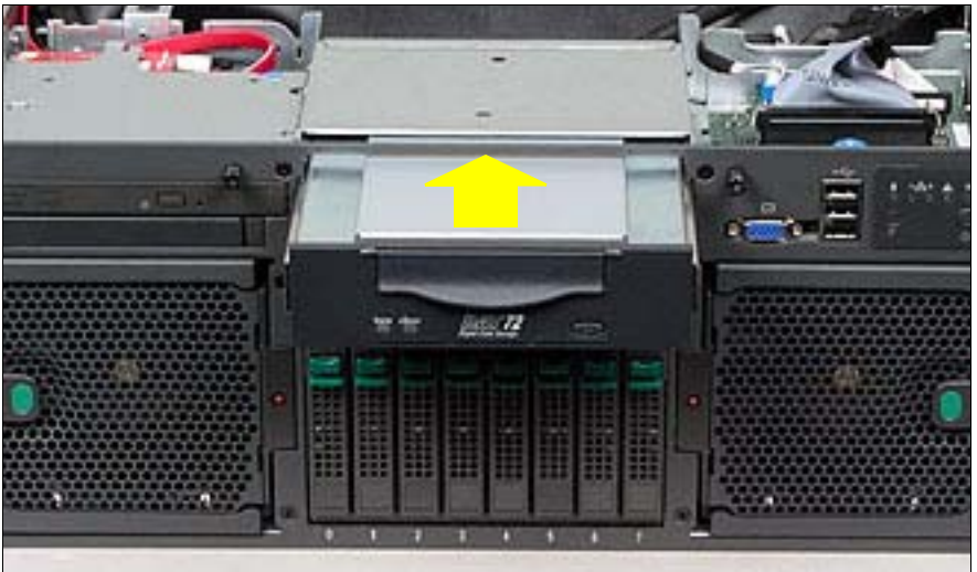
Figure 22: Inserting the tape drive
