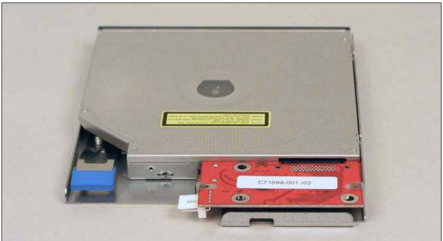
Figure 17: The pre-mounted CD/DVD drive (back)
