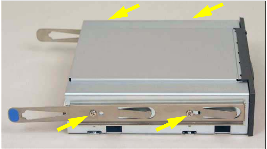
Figure 21: Fastening the sliding rails on the drive
