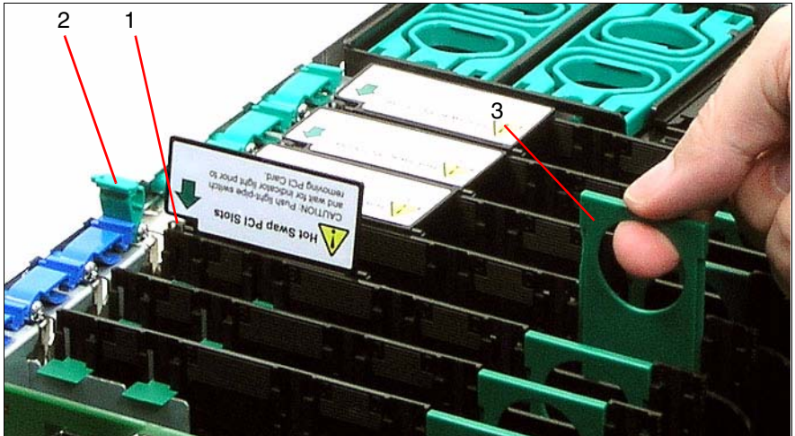
Figure 31: Deactivating, unlocking and removing the board
