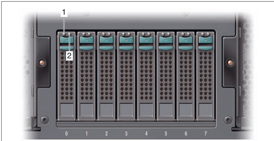
Figure 15: Indicators on an HDD module
