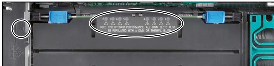
Figure 36: Example: Diagnostic LEDs on memory board B
