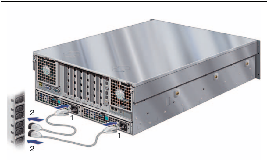
Figure 11: Connecting the server to the mains
