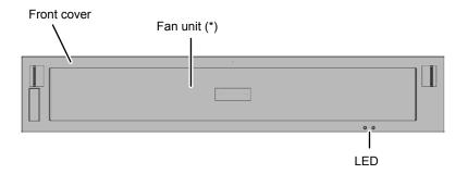
\*: You can see the fan unit by removing the front cover.
