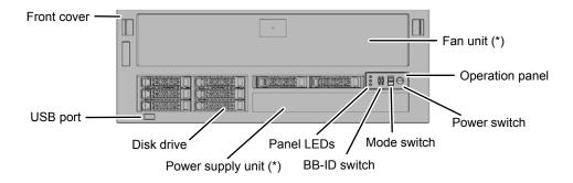
\*: You can see the fan unit and the power unit by removing the front cover.
