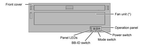
\*: You can see the fan unit by removing the front cover.
