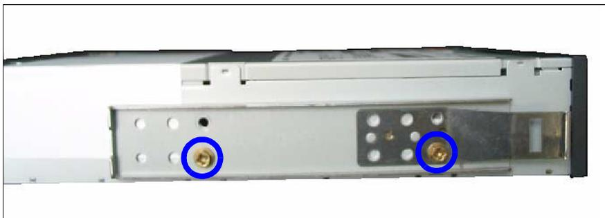
Figure 17: Attaching the EasyClick rails - magnetic tape drive LTO Ultrium 1HH
