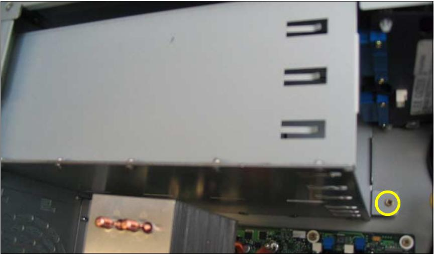
Figure 33: Fastening the PS cage in the housing
