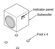
When the subwoofer is installed directly on flooring or a similar surface, fit the feet to the bottom of the subwoofer.
