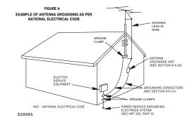
This reminder is provided to call the CATV system installer's attention to Article 820-40 of the NEC that
