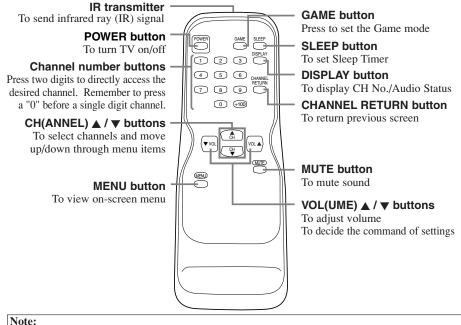
You can test if the remote control sends out the infrared signal with an AM radio. (Refer to "TROUBLESHOOTING GUIDE".)
