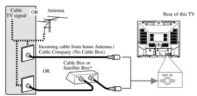
Incoming cable from Cable Company or Satellite Antenna
