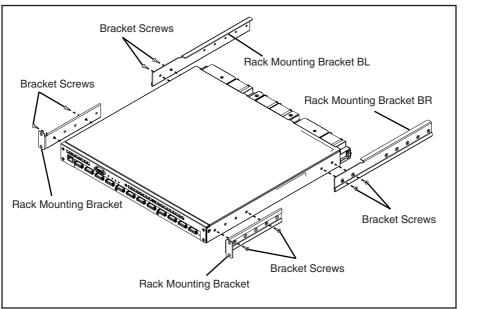
4. Slide the XG700 into the rack and fasten it in place.
