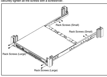
Securely tighten all the screws with a screwdriver.
