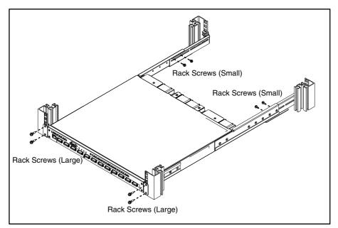
2. Slide the XG700 forward, and remove it from the rack.
