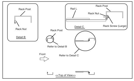
3. Fix the four rack mounting brackets to the XG700.
